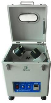
Step 2: Take out solder paste with the bushing (Tips: The bushing is not required if the diameter of the solder paste is larger than  $\Phi$  64), and take out the 500g balance code
