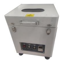
Step 5: Set the mixing time to reference 15 minutes (Tips:H is seconds, M is minutes, S is seconds), Time controller interface: set to 15M00
